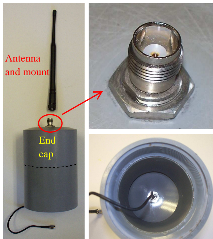
Figure 8. Antenna and mount on end cap (left), with close up view of mount (top right), and view looking inside the top (bottom right) with the antenna lead.
